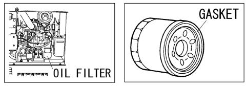
Loosen and remove the oil filter, using an oil filter wrench.
